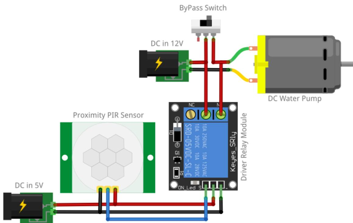
Gambar 3 Diagram wiring *hardware Automatic Sprayer Controller*
