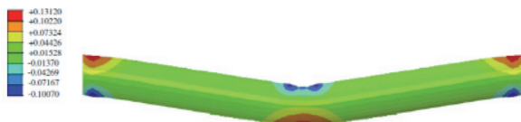
Figure 17: Plastic strain in steel section in case B
