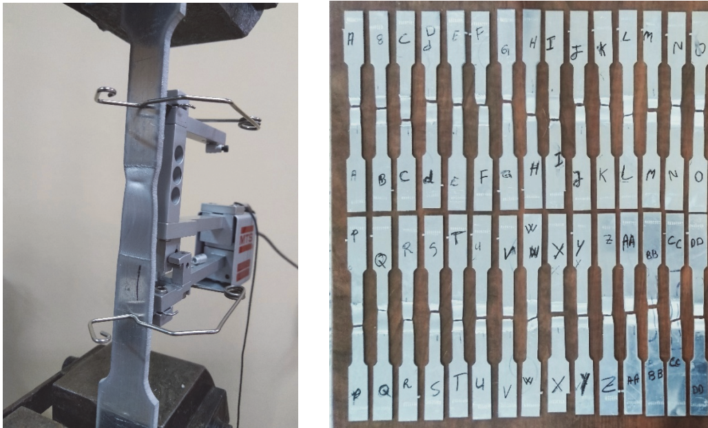
Figure 3: Dumbbell-shaped specimen tensile test measured by the extensometer
