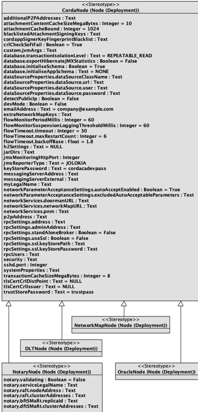
Fig. 5. UML Profile diagram presents stereotypes for nodes with tagged values.
