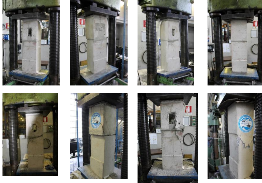
(a) (b) (c) (d) Fig. 4. Beginning (top) and end (bottom) of experimental tests on mockups: (a) additional cavity reinforcement and no mortar filling, (b) additional cavity reinforcement and mortar filling, (c) no additional cavity reinforcement and no mortar filling, (d) solid benchmark.
