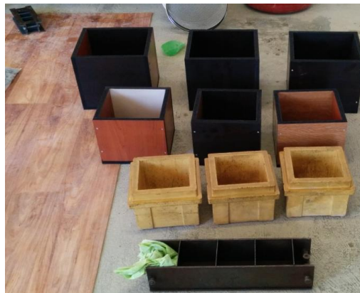
Fig. 1. The moulds prepared for each specimen size
