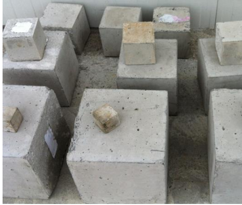
Fig. 2. Concrete specimens of 5 different sizes.
