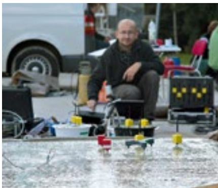
Interdisciplinary research at HTWK Leipzig: capillary pressure sensors for the aftertreatment of concrete, developed jointly by engineers at the Faculties of Civil Engineering and Electrical Engineering and Information Technology, help to prevent early damage. | Photo: Stephan Thomas
