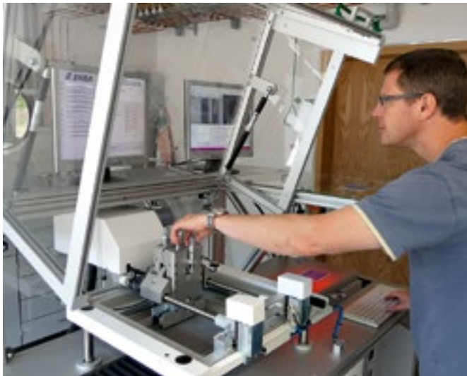
Manufacturing miniaturised sensors with the help of screen-printing technology at KSI Meinsberg.
