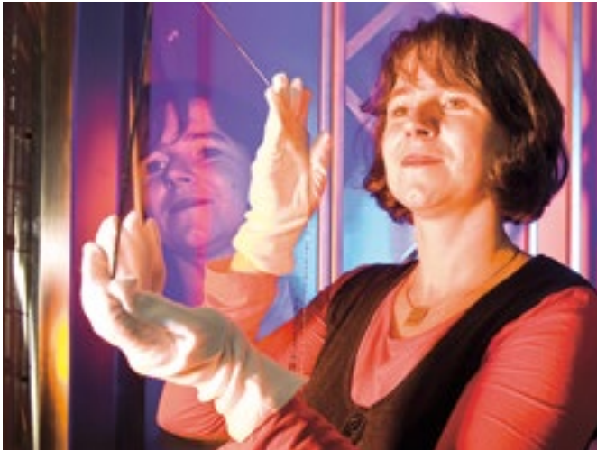
Glass substrate with transparent, conductive titanium dioxide coating – the electrode material of the future? | Photo: Fraunhofer FEP
