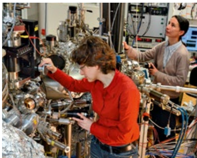
Ultrahigh vacuum facility for the production and study of thin layers. Photo: Steffen Giersch
