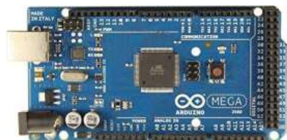
Gambar 7. Arduino MEGA 2560
