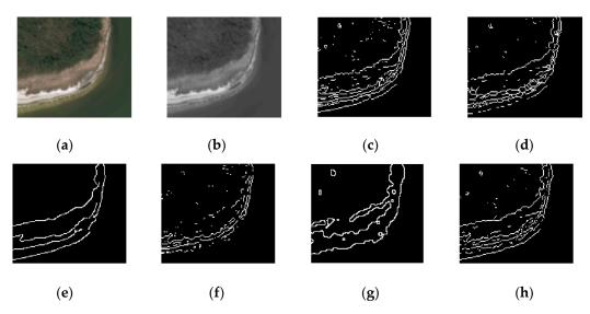
**Figure 14.** The region of satellite image "img6" after edge detection: (**a**) original color image (Landsat-7 image courtesy of the U.S. Geological Survey); (**b**) *Y* component of the original image; (**c**) Prewitt edge map; (**d**) Kirsch edge map; (**e**) Canny edge map; (**f**) LoG edge map; (**g**) morphological edge map; (**h**) SubPixel edge map.
