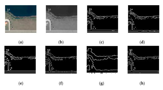
**Figure 9.** The region of satellite image "img1" after edge detection: (**a**) original color image (Landsat-7 image courtesy of the U.S. Geological Survey); (**b**) *Y* component of the original image; (**c**) Prewitt edge map; (**d**) Kirsch edge map; (**e**) Canny edge map; (**f**) LoG edge map; (**g**) morphological edge map; (**h**) SubPixel edge map.
