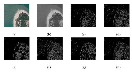
**Figure 11.** The region of satellite image "img3" after edge detection: (**a**) original color image (Landsat-7 image courtesy of the U.S. Geological Survey); (**b**) *Y* component of the original image; (**c**) Prewitt edge map; (**d**) Kirsch edge map; (**e**) Canny edge map; (**f**) LoG edge map; (**g**) morphological edge map; (**h**) SubPixel edge map.
