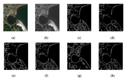
**Figure 12.** The region of satellite image "img4" after edge detection: (**a**) original color image (Landsat-7 image courtesy of the U.S. Geological Survey); (**b**) *Y* component of the original image; (**c**) Prewitt edge map; (**d**) Kirsch edge map; (**e**) Canny edge map; (**f**) LoG edge map; (**g**) morphological edge map; (**h**) SubPixel edge map.
