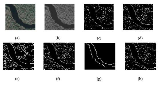
**Figure 13.** The region of satellite image "img5" after edge detection: (**a**) original color image (Landsat-7 image courtesy of the U.S. Geological Survey); (**b**) Y component of the original image; (**c**) Prewitt edge map; (**d**) Kirsch edge map; (**e**) Canny edge map; (**f**) LoG edge map; (**g**) morphological edge map; (**h**) SubPixel edge map.
