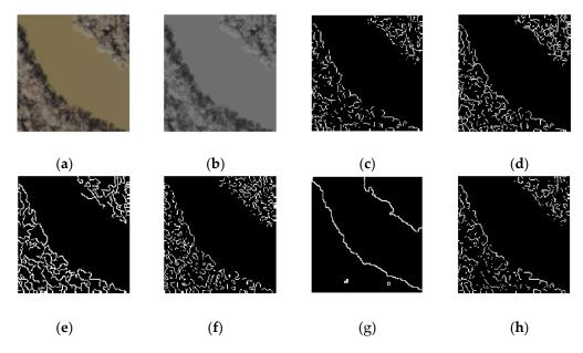
**Figure 10.** The region of satellite image "img2" after edge detection: (**a**) original color image (Landsat-7 image courtesy of the U.S. Geological Survey); (**b**) *Y* component of the original image; (**c**) Prewitt edge map; (**d**) Kirsch edge map; (**e**) Canny edge map; (**f**) LoG edge map; (**g**) morphological edge map; (**h**) SubPixel edge map.
