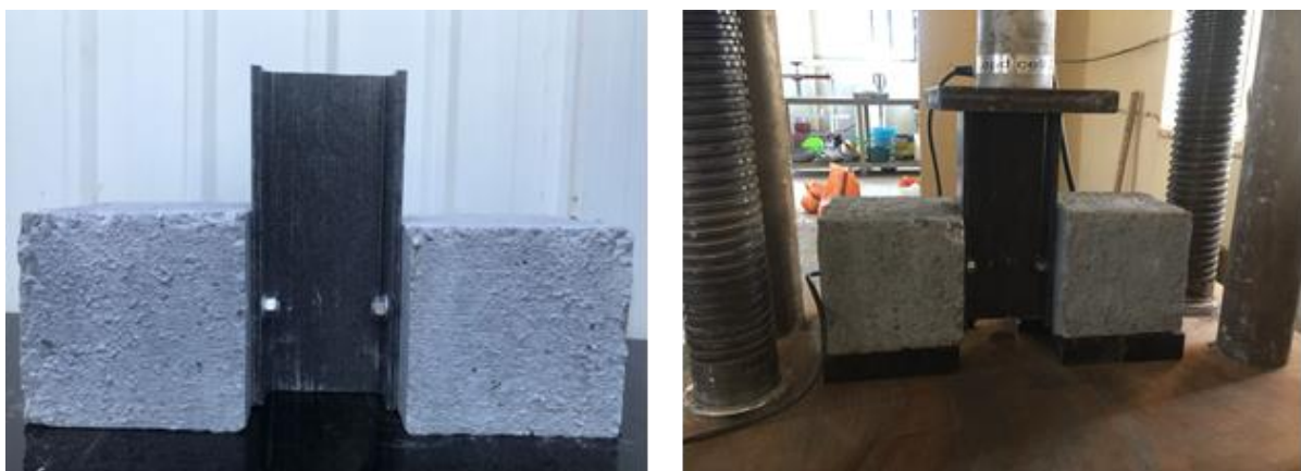
Figure 5. Shear connection test setup
