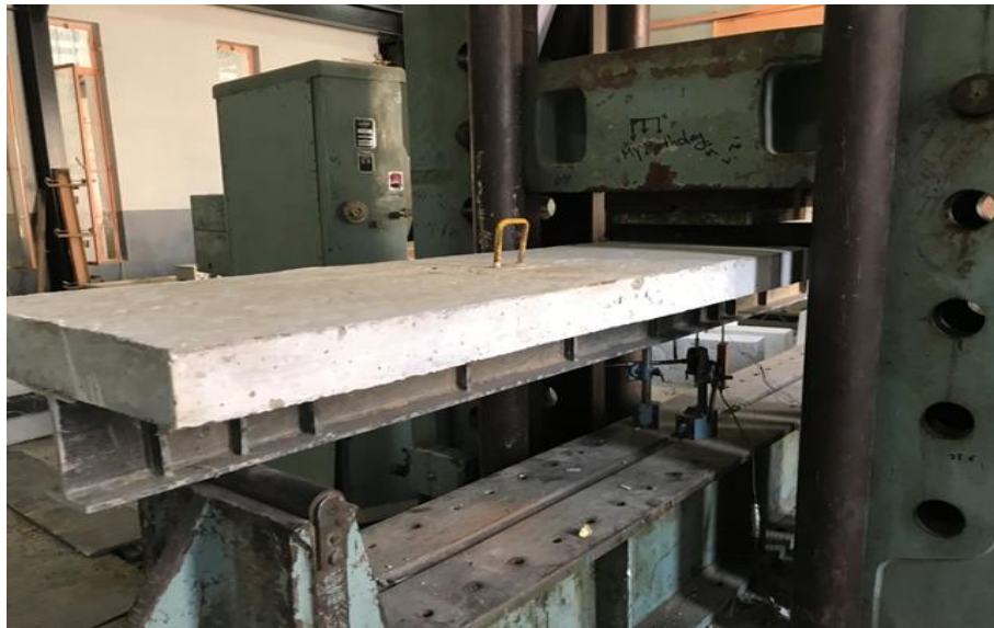
Figure 8. Flexural test setup—hybrid beam
