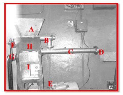
Figure 2: Picture of the extruder
