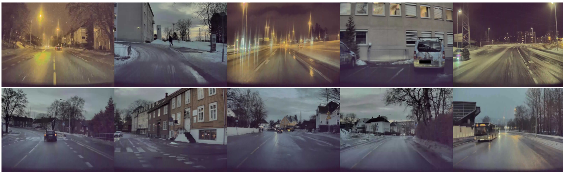
Figure 15: Images selected from the Trondheim-area by only using Model-B: Fully trained CityScapes model from Detectron2 (Mask R-CNN). 15a : Top 10 hard images starting with the hardest. 15b : Top 10 easy images starting with easiest.
