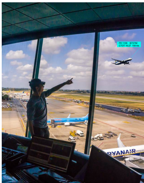
Fig. 1 An operator wearing a head-mounted see through display in the control tower can see information superimposed to the real out of the tower view. In the example it is shown a label for taking off flight identification and status with alphanumeric dynamic text labels
