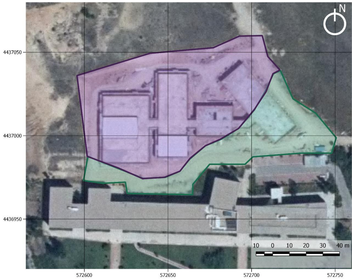
Figure 7. Distribution of the cut-off (purple) and fill (green) areas on the plot where the building is located.
