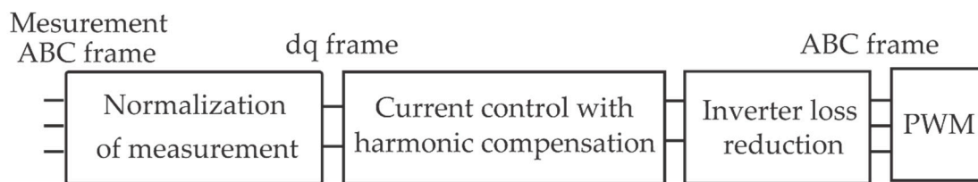
Figure 5. Detailed view of the control system of the VSC of HRES.
