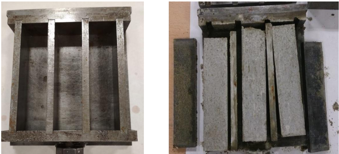
Fig. 1. Mortar specimens production according to UNE-EN 12504-1:2009
