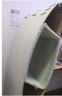
Fig. 1.4 Wind turbine’s blade employed in the experiments
