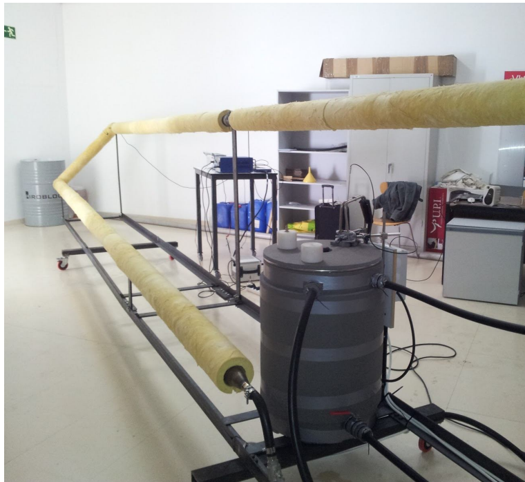
Fig. 1.3 Test rig: austenitic stainless steel pipes
