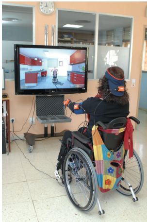
FIGURE 2: Virtual reality system Toyra. Arm movements are captured by Inertial Sensors Xsens (Xsens Inc., Netherlands). An avatar represents in real time and mirror view the movements of the user performing a task in the virtual scenario.
