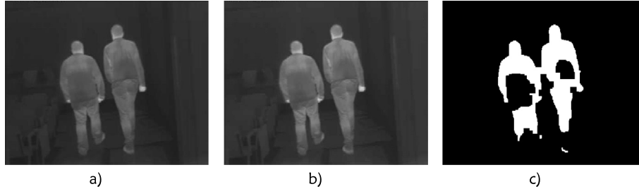
Fig. 2. (a) Input IR image frame. (b) Scaled frame. (c) Closed soft threshold.
