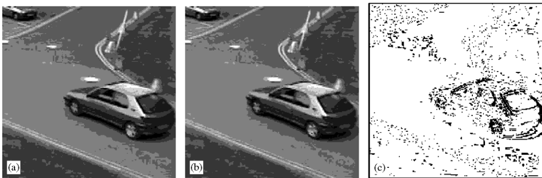
Fig. 2. (a) Image segmented into eight gray level bands at t - 1 ; (b) image segmented into eight gray level bands at t ; (c) motion presence at t .
