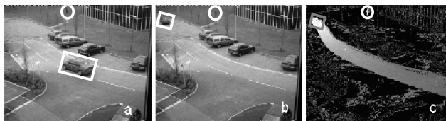
Fig. 1. Motion charge map: (a) one image of a sequence, (b) same perspective after some seconds, (c) motion trails as represented on the bidimensional motion charge map
