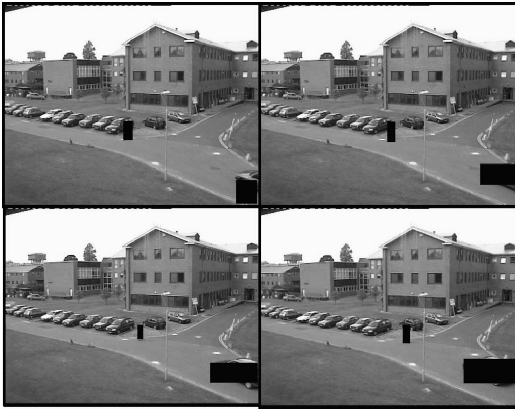
Fig. 11. Car and pedestrian fuzzy regions for images 61, 73, 85 and 98 of the second example.
