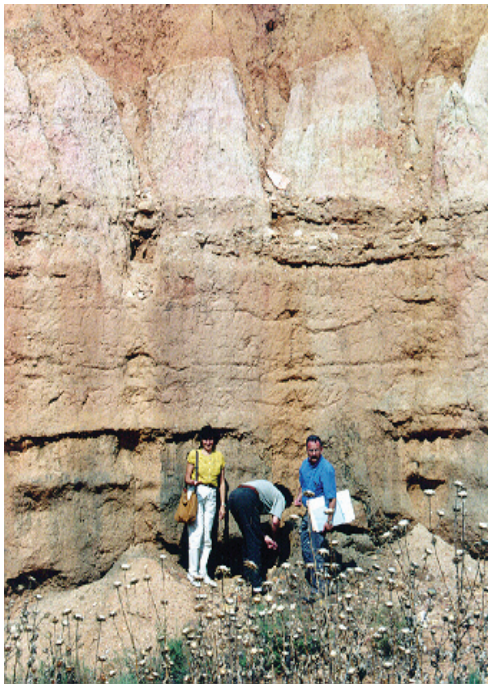
Figure 18. El Chorrillo mine. The dark level, coinciding with the person's highness, corresponds to the orebody thickness.
