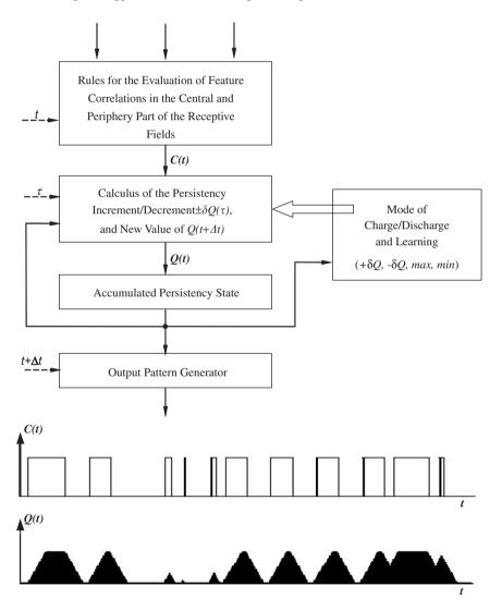
Fig. 13. The AC inferential schema (upper part) and an example of the temporal evolution of the accumulated persistency state, Q(t), in response to a specific sequence of values of a detected feature, C(t), (lower part).
