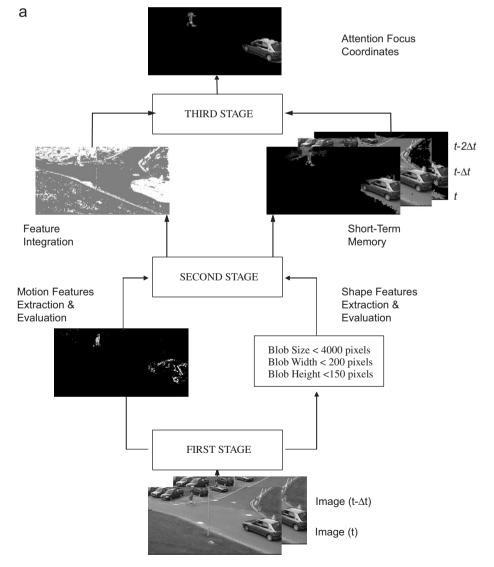
Fig. 7. Results of the bottom-up and top-down organizations in a surveillance scenario. (a) Bottom-up. (b) Top-down.
