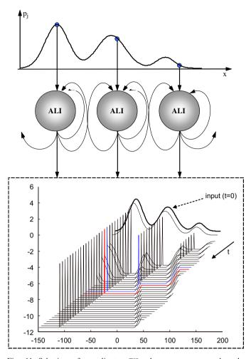
Fig. 11. Selection of coordinate  $x_j^{\text{max}}$  where property  $p_j$  takes the maximum value in the time interval considered. Result of the simulation after 30 iterations and convergence in the maximum value starting from iteration 12, with 201 calculation units and a receptive field of 11 units (1 central and 10 peripheral). The coordinate where the value of  $p_j$  is maximum is x = 41.
