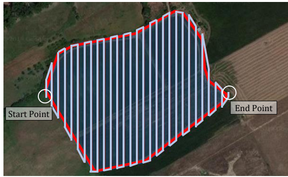
Figure 6: Perimeter of the polygon to be inspected. In red, the optimal route that the UAV will follow within the polygon to obtain multispectral images.
