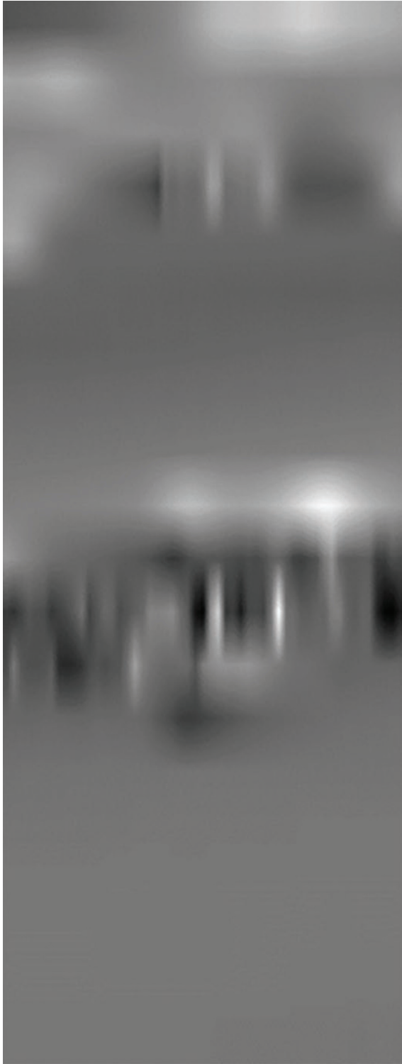
Figure 1. Example of a spectral record represented as a grayscale image. Mid-infrared spectral images were created by reshaping spectral records from an array of size 1,060 \times 1 to an array of size 53 \times 20 . Each wavelength value in the reshaped array was normalized (in the range 0–1), multiplying by 255 to represent the wavelength values as grayscale pixels, and saved as a PNG image. Image filenames were generated using label, animal, and sample information. These spectral images were then used as features in training the deep neural networks.
