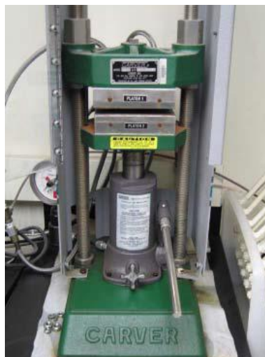
Figure 11: GDL is applied to the membrane in the hot press [42]
