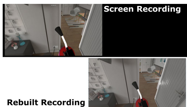
Fig. 1 Screenshot captured from video comparison showing real-time video capture of a simulation and rebuilt capture using Virtual Observation. The full video can be viewed here: https://www.youtube.com/watch?v=2YY-d7QMUVI . The Virtual Observation system can be included in any SteamVR compatible Unity project by adding the VO component to the default VR camera rig set-up and linking the input states of the developers/researchers interaction system (so the actions can be recorded and later replicated). Recorded data can be stored in XML or JSON file formats and supports all VR headsets and tracked controllers that are compatible with SteamVR and the Unity game engine
