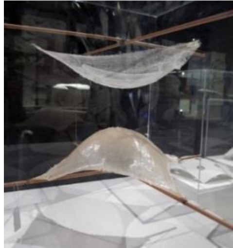
Figure 16. Hanging fabric and inverting its form for thin shells by Isler. (Source: designboom.com)
