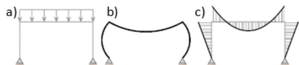
Figure 38. Finding optimum form of portal frame not using single-bay catenary: a) A given portal frame; b) Deformation of frame under the load; c) Bending moment diagram of frame
