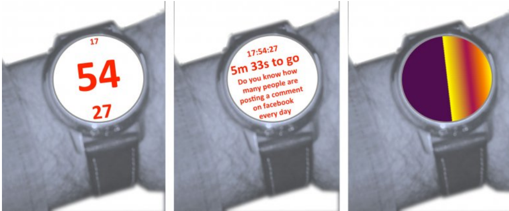
Figure 2.1: Design sketches that illustrate time visualisations in different contexts. (a) For users running to catch a bus, making it easy to see the minutes in large fonts. (b): For boring lectures and meetings, showing a countdown to the end, with some information to engage the user. (c) Visualisation giving only a very coarse idea of the time, similar to information you get from the sun, to use for example when hanging out with friends when time does not matter (Schmidt 2013 )
