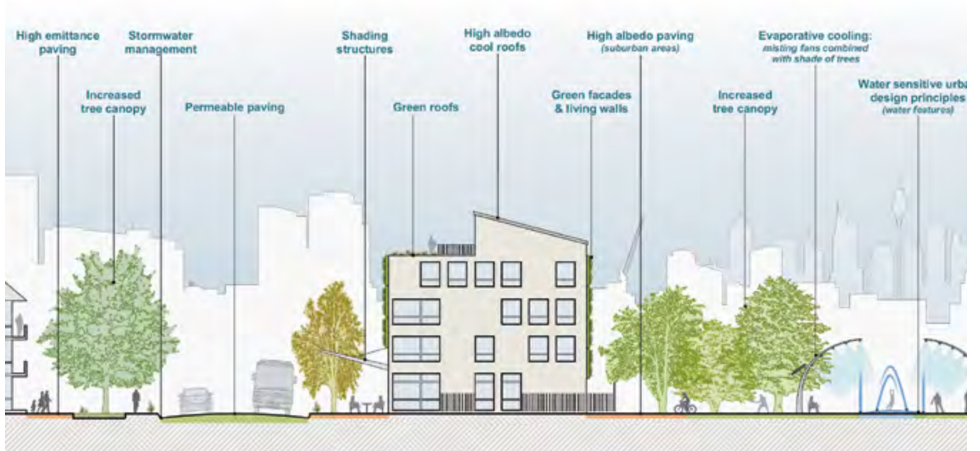
Figure 23: Urban design strategies for cooler cities. Source: RP2024 Guide to Urban Cooling Strategies 2017 (Low Carbon Living CRC, 2017). Retrieved from http://www.lowcarbonlivingcrc.com.au
