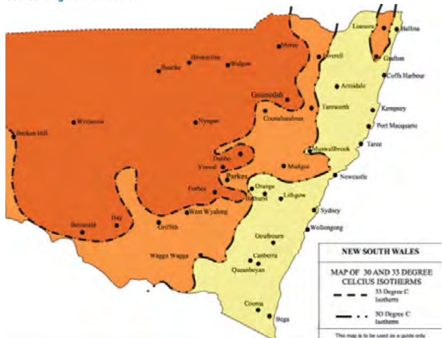
Figure 12: Identification of zones in NSW based on mean maximum January isotherms. Source: efsg.det.nsw.edu.au
