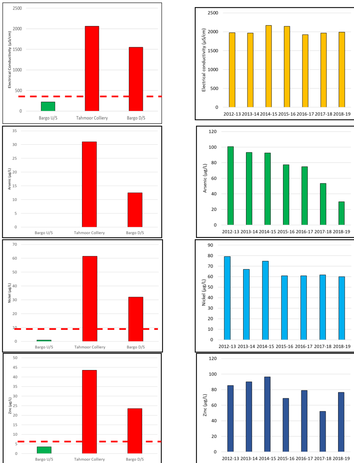
Figure 2. Mean water quality results collected from the current study (graphs on the left) for salinity (i and ii), arsenic (iii, iv), nickel (v, vi) and zinc (vii and viii). The mean values in the current study are for Bargo River upstream (U/S), Tahmoor Colliery waste and Bargo River downstream (D/S). The graphs on the right are the mean annual values (2012/3 to 2018/9) for these four pollutants in Tahmoor Colliery waste discharges [6]. The dotted red lines represent the ANZECC [7] guideline values for protection of aquatic species.
