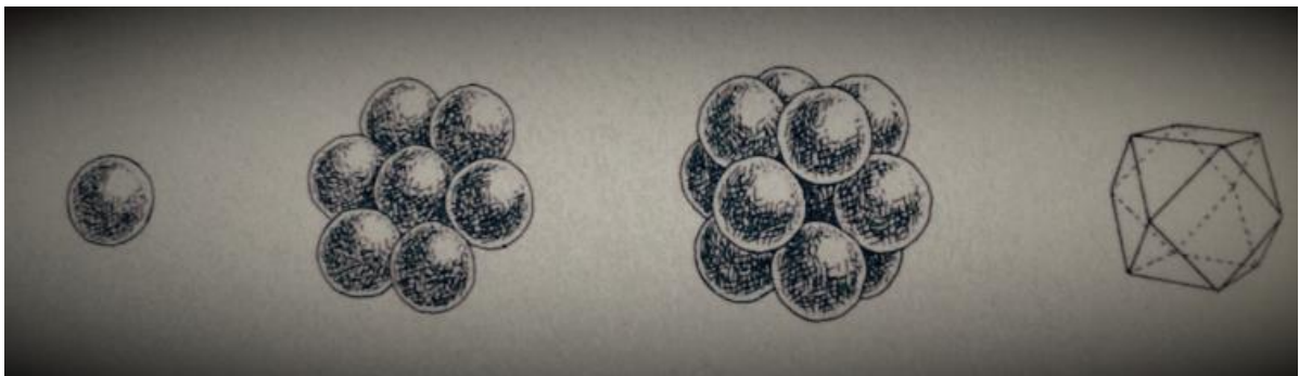
Figure 5. Formation of a cuboctahedron and crystallisation. 23
