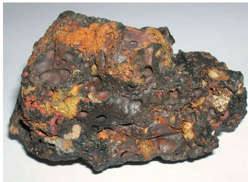
Figure G1: Lump of slag from iron smelting
