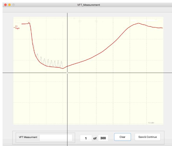
Figure A.1. VFT annotation GUI opened. A cursor is available for selecting the start point of refilling.
