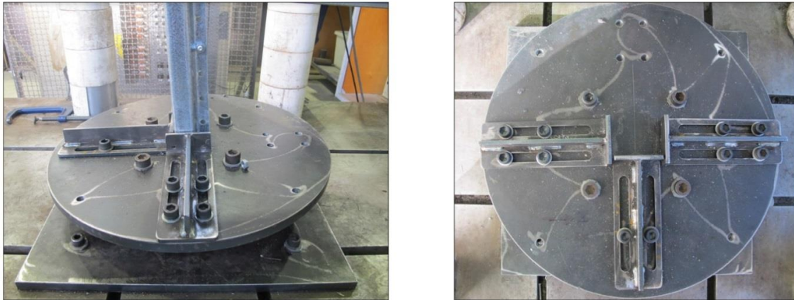
Figure 9. Adjustable cap connection supports.
