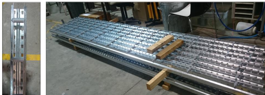
Figure 5. Reinforcement along the upright length by bolts and spacers.
