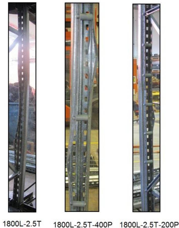
Figure 13. Failure modes of upright frames with 2.5 mm thickness.
