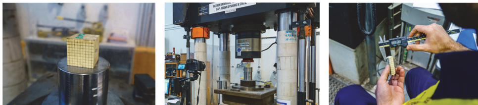
Fig. 4. Loading test for determining the compressive properties of selected foam
