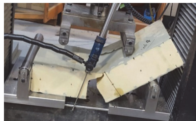
Fig. 9. Bending test of created system specimen
