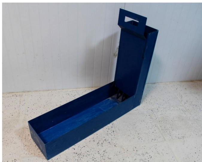
Figure 8. The L-box setup for workability measurement.
