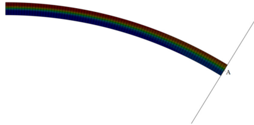
Figure 10. Finite element modelling of the pure bending of the metal sheet sample.
