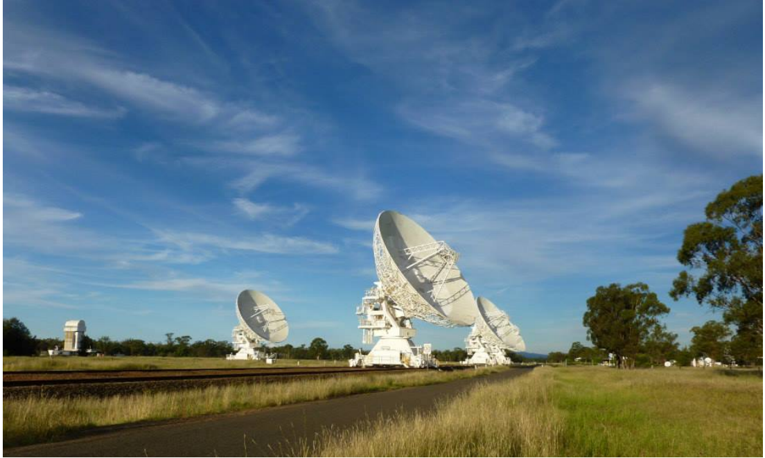
Figure 2.2: Four of the six 22-m dishes that make up the ATCA radio interferometer. Image has been used with permission from Graeme Wong.
