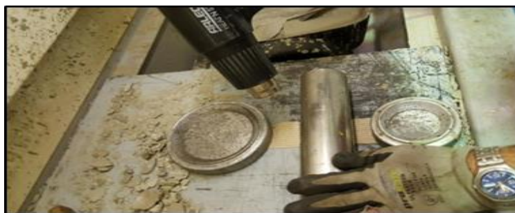
Figure 3.9: Heat-welded specimens of Barrateen fabric
