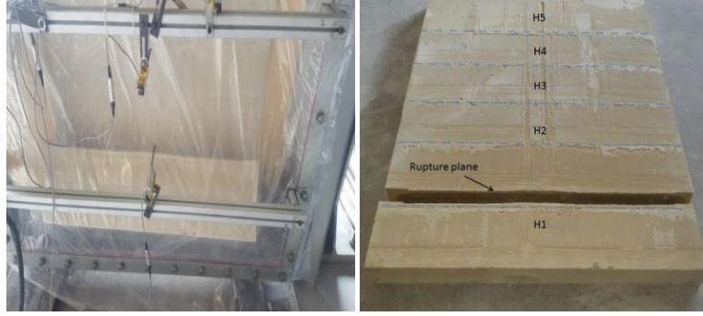
Fig10. Typical collapse mode of TS panels at seam H1 under monotonic loading (test series 2)
