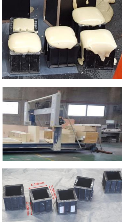
Figure 5.2: Empty cubic formworks (bottom) and foam filled ones (top) before been machined (mild)
