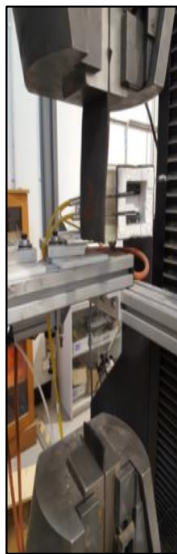
Figure 3.6: Brittle behaviour of Rubber fabric specimens
