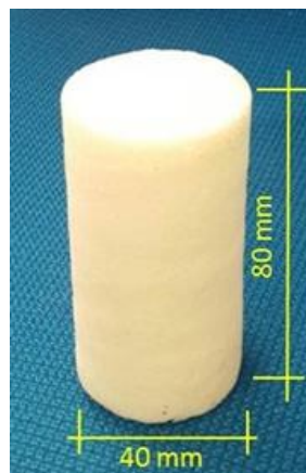
Figure 5.1: Obtained cylindrical specimens for density test
