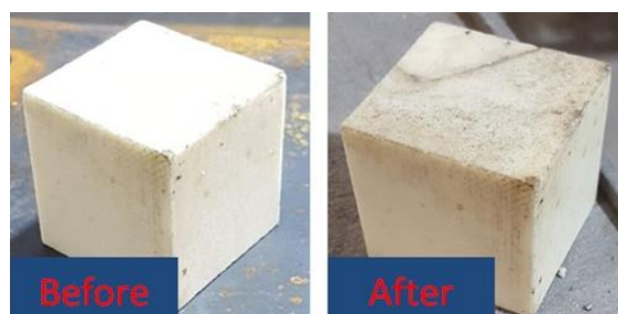
Figure 5.3: Minor darkening of specimens at 72 °C after 836 hours
