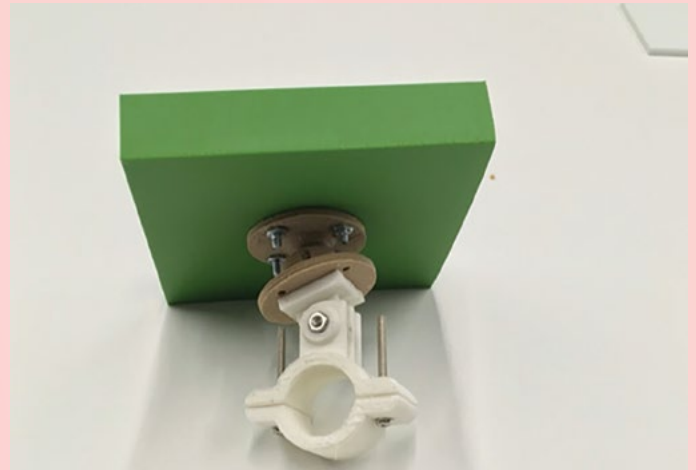
1st version 3D printed smartphone holder with wheelchair mount
