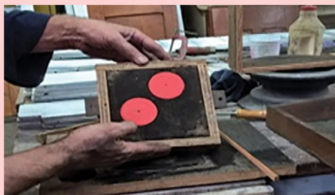
Top: 3D printed positive, wax cast and silicon mould. Bottom: Sand casting experiment with 3D prints.
