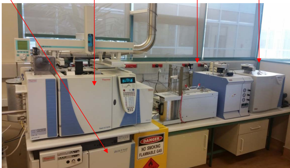
Figure 2.8: The Thermo Fisher Scientific Flash 2000 Organic Elemental Analyzer coupled with a Thermo Fisher Scientific Finnigan Delta-V Isotopic Ratio MS.
