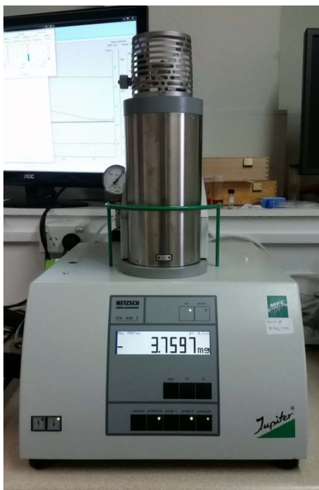
Figure 2.7: The NETZSCH STA 449C Jupiter Thermos-Balance used for asphaltene profiling.
