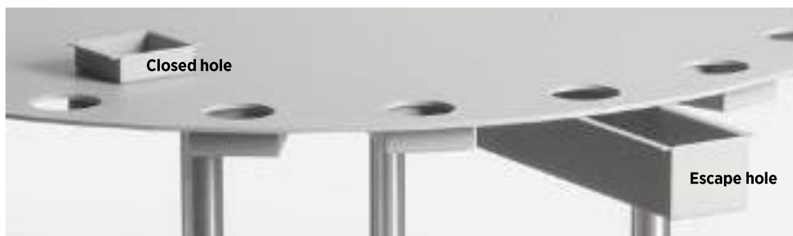
Fig. 6 Showing the closed hole and escape hole brackets. The escape hole bracket is replaced with a closed hole bracket during the probe trial.
