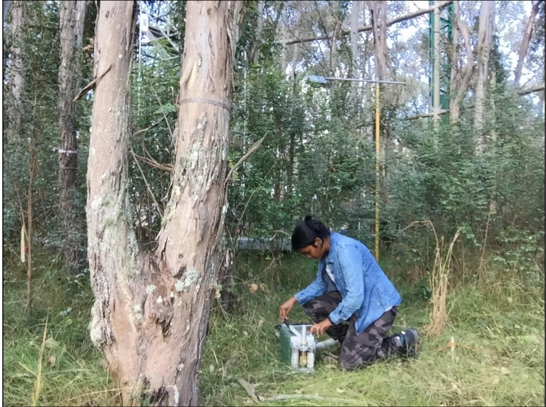
Image 2.1 Photosynthetic gas exchange measurements, using a LiCOR-6400 at the EucFACE.
