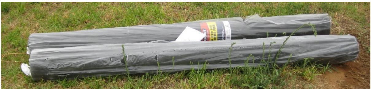
Figure A.4: Heavy duty polythene sheets (100 microns) used to prevent salt leaching to the soil.
