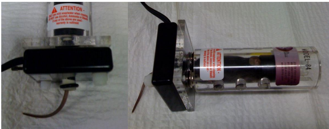
Figure 3.4.1: Mouse in the Perspex restrainer showing tail cuff and sensor
