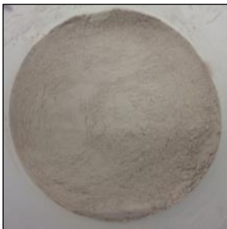
Figure 3.4: Dried at 130°C, \text{LiMnPO}_4 precursor material produced with stoichiometric amounts of lithium, manganese and phosphorous chemicals. The material was ground at 400 rpm for 1 hour to produce a fine powder.
