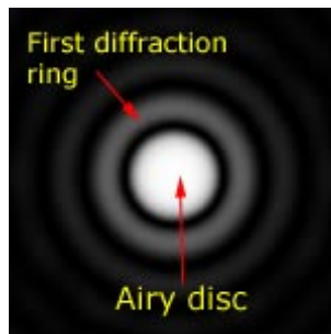
Figure 1.4: An Airy disc, showing the main lobe and diffraction fringes (or side lobes) formed by a circular aperture. Image provided by Brian Burton, Boston University.
