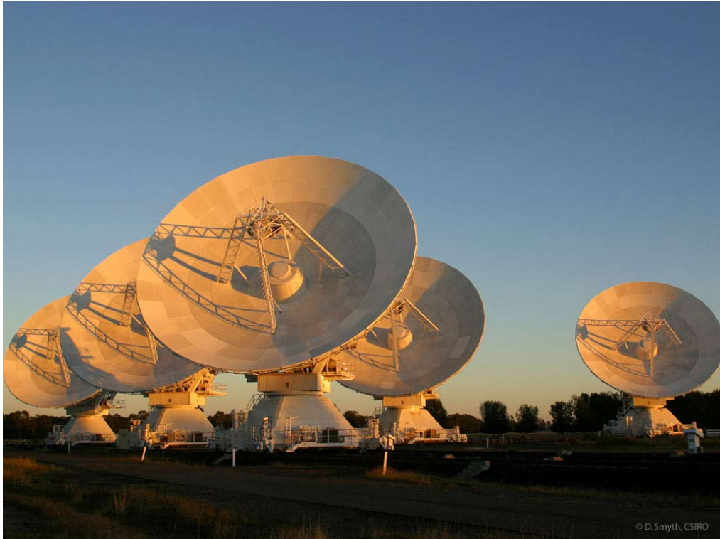
Figure 1.6: The Australia Telescope Compact Array (ATCA), an interferometer in Narrabri, northern NSW. Image courtesy of CSIRO.
